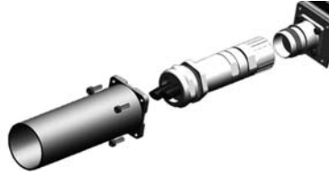
Figure 9: Fitting the protective sleeve (option)
