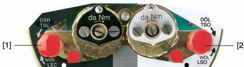
1. Turn test button [1] in direction of the TSC arrow: Torque switch CLOSED trips.
