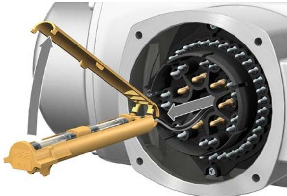
2. Pull fuse holder out of pin carrier, open fuse cover and replace old fuses by new ones.
