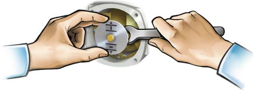
2. Refer to table and check if turns/stroke of the actuator correspond to the setting of the reduction gearing (stages 1– 9).
