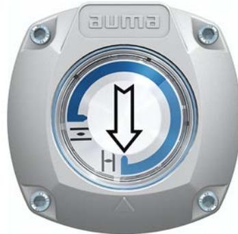
The self-adjusting mechanical position indicator shows the valve position by means of an arrow  $\Rightarrow$ . When correctly set, the arrow points to symbol  $\equiv$  (OPEN) or  $\perp$  (CLOSED) in the end positions.
