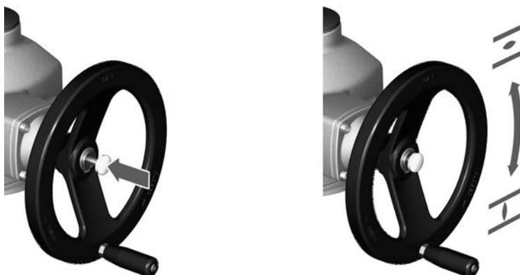
➔ The closing direction is marked on the handwheel.
