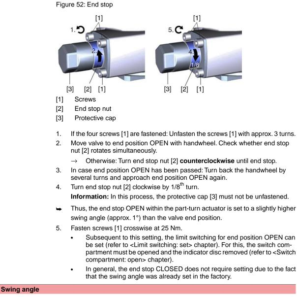
The swing angle must only be changed if the swivel range for end stop setting is not sufficient.
