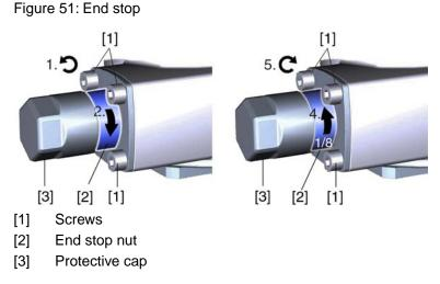
1. If the four screws [1] are fastened: Unfasten the screws [1] with approx. 3 turns.
