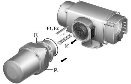
2. Pull fuse holder [3] out of pin carrier, open fuse cover and replace old fuses by new ones.
