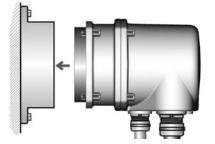
Figure 20: Parking frame and plug/socket connector with terminal blocks (KES)
