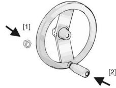
3. After ball handle fitting, remove label from handwheel.
