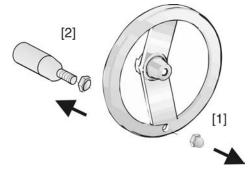
2. Insert ball handle [2] in correct position and fasten with cap nut [1].
