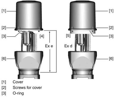
Figure 14: Plug/socket connector: left KES, right KES flameproof
