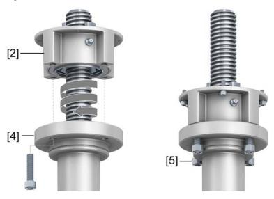
6. Fit multi-turn actuator on the valve stem so that the stem nut dogs engage into the output drive sleeve.
