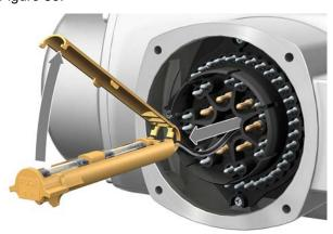
2. Pull fuse holder out of pin carrier, open fuse cover and replace old fuses by new ones.
