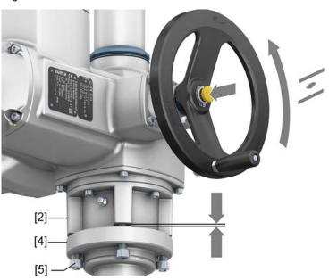
11. Tighten screws [5] between valve and output drive type A crosswise applying a torque according to table.
