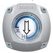
The self-adjusting mechanical position indicator shows the valve position by means of an arrow  $\Longrightarrow$ . When correctly set, the arrow points to symbol  $\stackrel{\blacksquare}{=}$  (OPEN) or  $\stackrel{\blacksquare}{\perp}$  (CLOSED) in the end positions.
