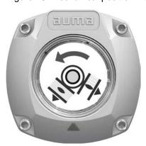
The mechanical position indicator shows the valve position via two indicator discs with symbols  $\subseteq$  (OPEN) and  $\boxed{\bot}$  (CLOSED). When correctly set, the symbols OPEN/CLOSED point to the indicator mark  $\blacktriangle$  at the cover in the end positions.
