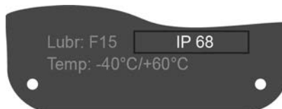
Figure 32: Name plate, example with enclosure protection IP68
