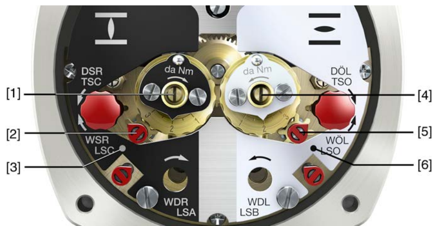
Figure 85: Setting elements for limit switching
