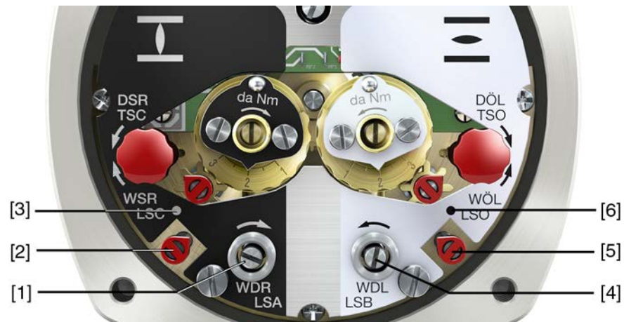
Figure 86: Setting elements for limit switching
