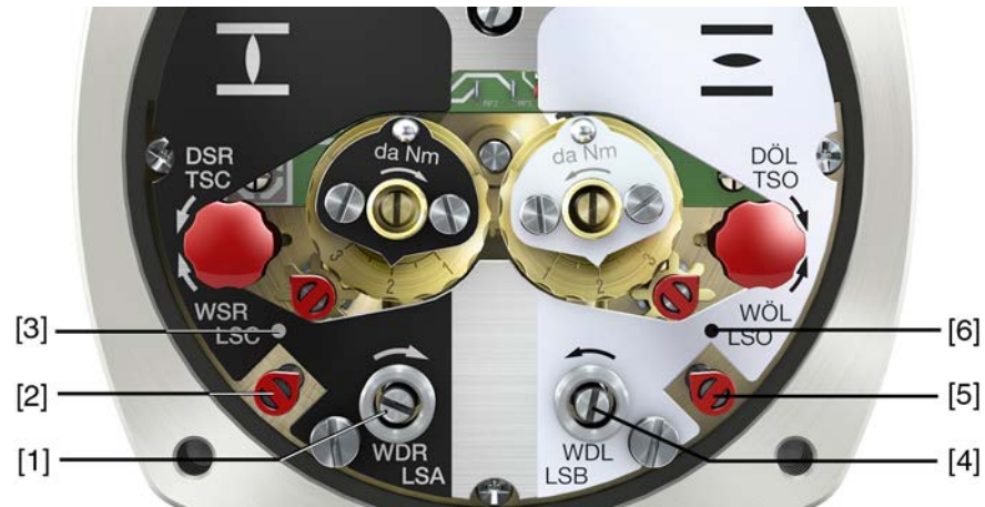
Figure 90: Setting elements for limit switching
