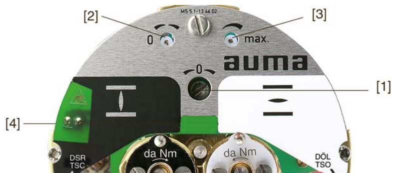
Figure 89: View on control unit when switch compartment is open
