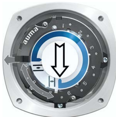
Figure 76: Set reduction gearing
