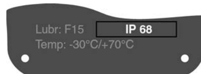
Figure 25: Example: Name plate for enclosure protection IP68
