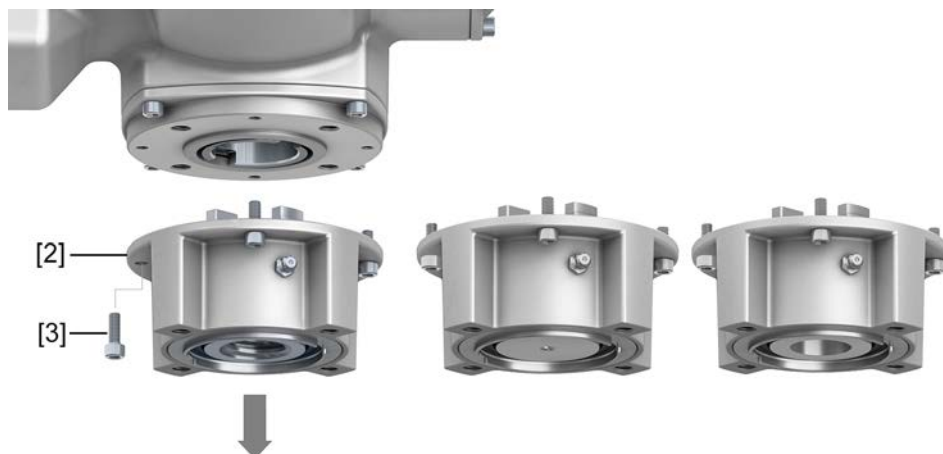
Figure 12: Multi-turn actuator with output drive type A
