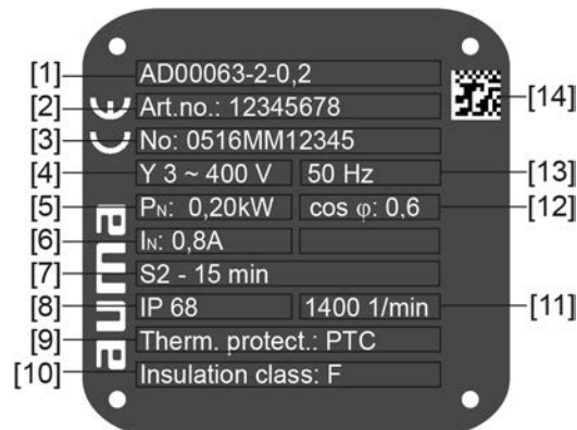
Figure 7: Motor name plate (example)
