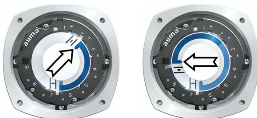
Figure 75: Operation in direction OPEN (left) and position OPEN (right)
