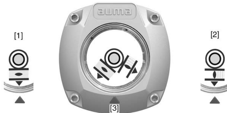
Figure 67: Mechanical position indicator
