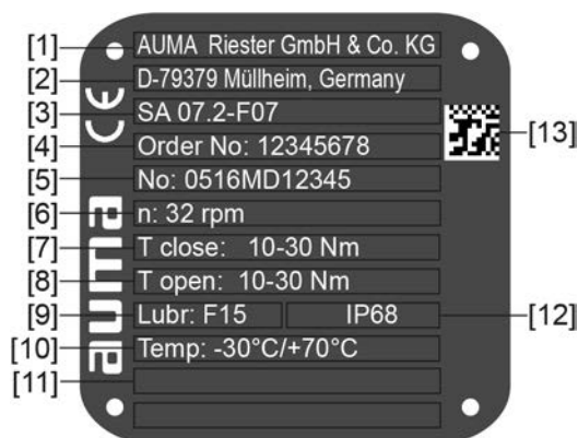
Figure 5: Actuator name plate (example)
