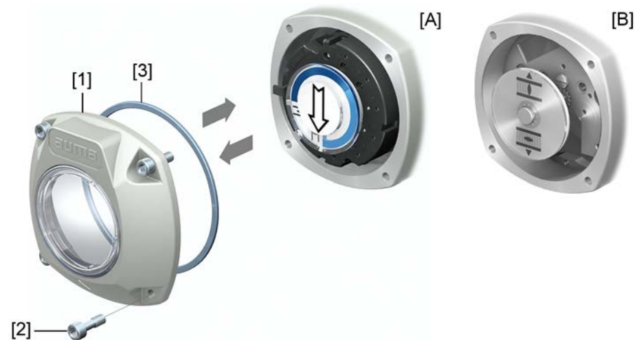
Figure 72: Open/close switch compartment
