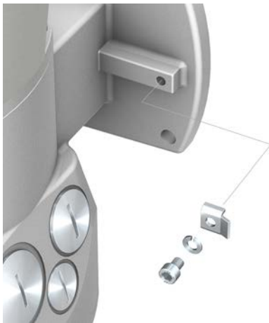
Figure 40: Earth connection for wall bracket
