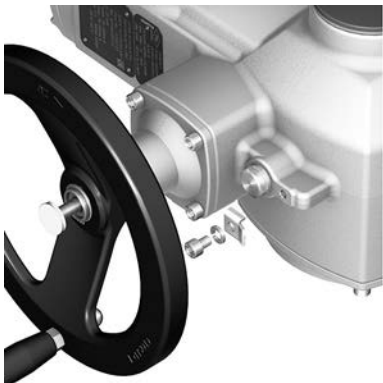
Figure 37: Earth connection for multi-turn actuator
