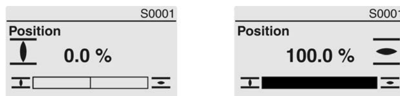
Figure 54: End position CLOSED/OPEN reached
