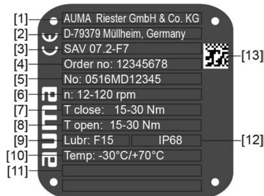
Figure 5: Actuator name plate (example)
