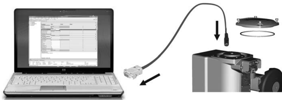
Figure 26: Connection with service cable
