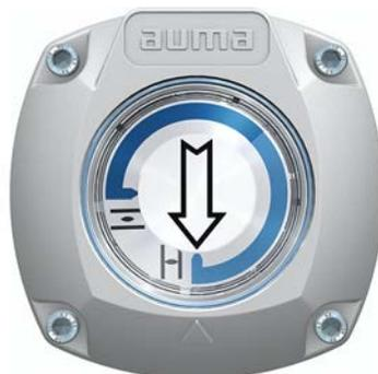
The self-adjusting mechanical position indicator shows the valve position by means of an arrow  $\Downarrow$ . When correctly set, the arrow points to symbol  $\equiv$  (OPEN) or  $\perp$  (CLOSED) in the end positions.
