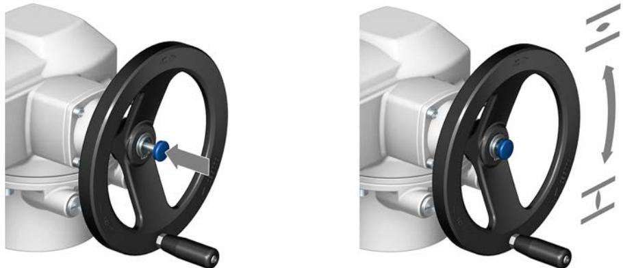
↳ The closing direction is marked on the handwheel.
