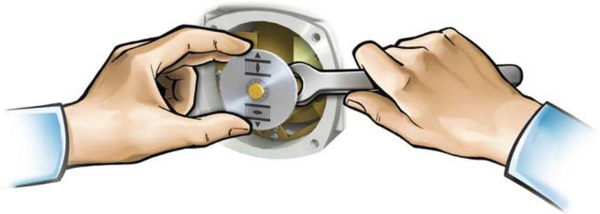
2. Refer to table and check if swing angle of the actuator corresponds to the setting of the reduction gearing (stages 1– 9).
