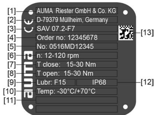
Figure 5: Actuator name plate (example)
