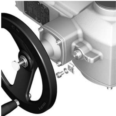
Figure 37: Earth connection for multi-turn actuator
