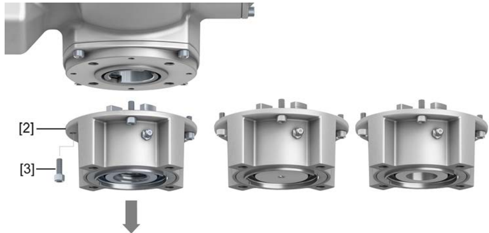
Figure 13: Multi-turn actuator with output drive type A
