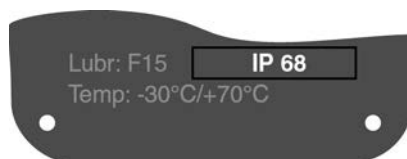
Figure 31: Example: Name plate for enclosure protection IP68
