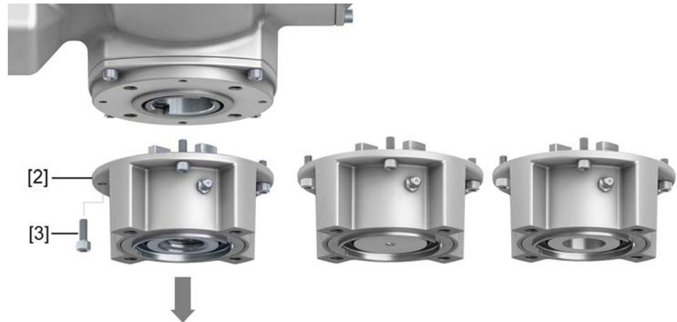
Figure 13: Multi-turn actuator with output drive type A
