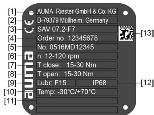
Figure 5: Actuator name plate (example)
