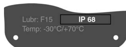
Figure 23: Example: Name plate for enclosure protection IP68
