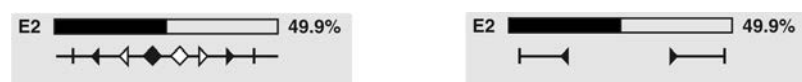
Figure 48: Examples: on the left pivot points (intermediate positions); on the right stepping mode
