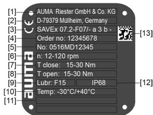
Figure 5: Actuator name plate (example)
