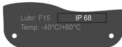
Figure 32: Name plate, example with enclosure protection IP68
