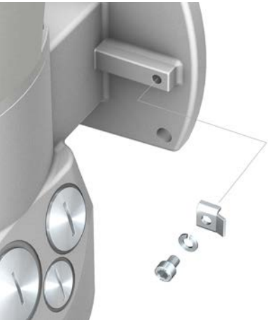
Figure 41: Earth connection for wall bracket
