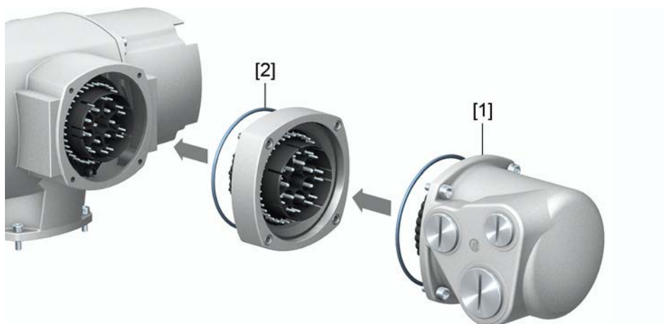
Figure 31: Electrical connection with DS intermediate frame
