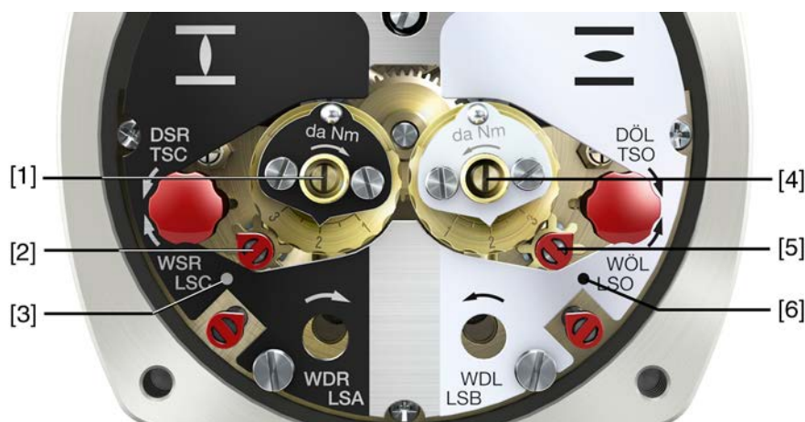
Figure 63: Setting elements for limit switching
