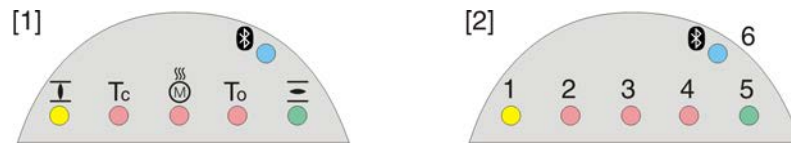
Figure 72: Arrangement and signification of indication lights
