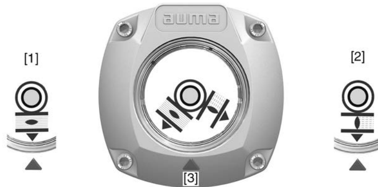
Figure 76: Mechanical position indicator
