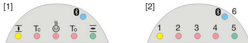
Figure 75: Arrangement and signification of indication lights
