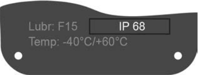
Figure 34: Name plate, example with enclosure protection IP68
