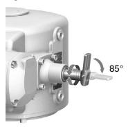
2. Push handwheel over the red change-over lever then onto the shaft. Figure 11:
