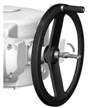
3. Release change-over lever (should snap back into initial position by spring action, if necessary, push it back manually).
