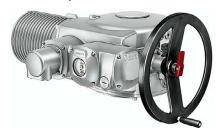
AUMA multi-turn actuators SA 25.1-SA 48.1/SAR 25.1-SAR 30.1 are driven by an electric motor and are capable of withstanding thrust in combination with output drive type A. For manual operation, a handwheel is provided. Switching off in end positions may be either by limit or torque seating. Actuator controls are required to operate or process the actuator signals.
