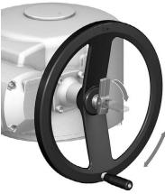
Release change-over lever (should snap back into initial position by spring action, if necessary, push it back manually).
