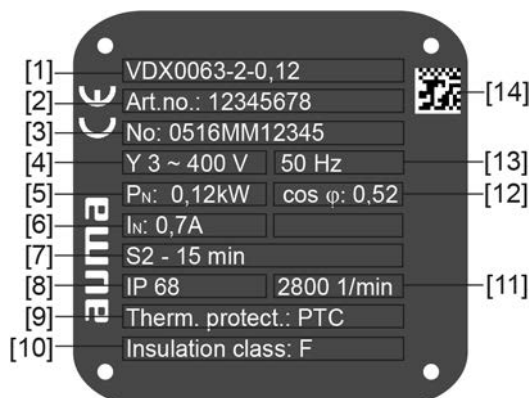
Figure 6: Motor name plate (example)
