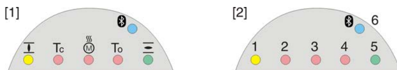
Figure 62: Arrangement and signification of indication lights
