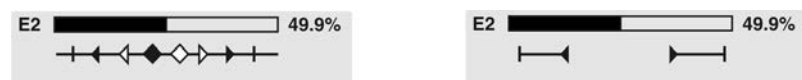
Figure 43: Examples: on the left pivot points (intermediate positions); on the right stepping mode
