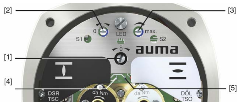
Figure 66: View on control unit when switch compartment is open
