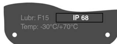
Figure 23: Example: Name plate for enclosure protection IP68
