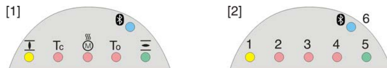
Figure 55: Arrangement and signification of indication lights
