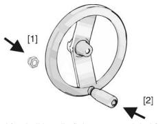
3. After ball handle fitting, remove label from handwheel.
