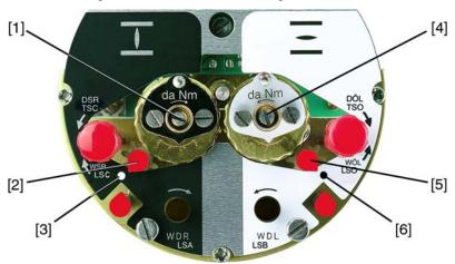
Figure 67: Setting elements for limit switching
