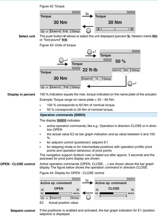
The direction of the operation command is displayed by an arrow above the bar graph indication. The figure below shows the operation command in direction CLOSE.
