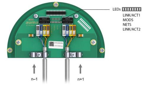
Figure 23: Profinet connection board with connection terminals
