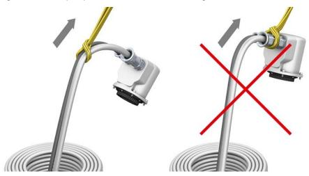
Figure 14: Minimum bending radii at plug/socket connector of actuator
