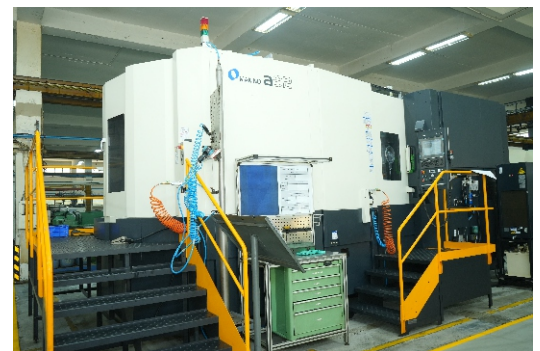
Makino A92 HMC capable of machining components up to 1.2 x 1.8 x .5 (LxWxH) metres in size
