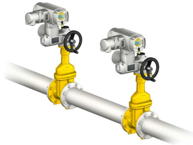
Figure 5: Redundant system with Safe ESD for Safe OPENING
