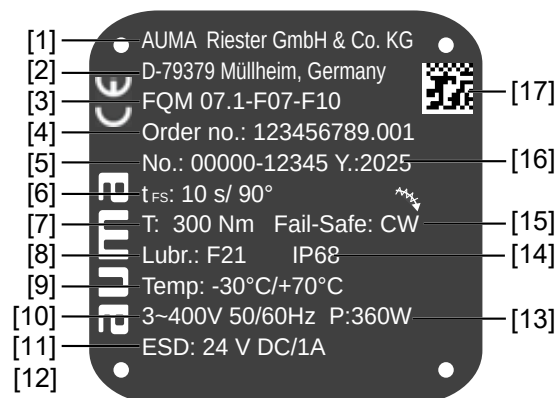
Figure 3: Fail safe unit name plate (example)
