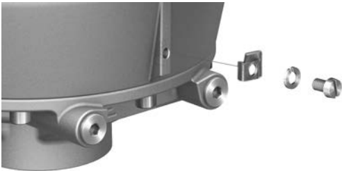
Figure 21: External earth connection
