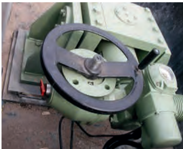
Figure 3.21: Horizontal handwheel offset by 90° in front of an actuator
