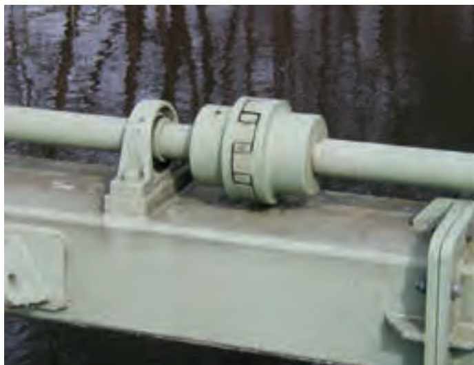
Figure 2.056: Elastic safety coupling for torque transmission
