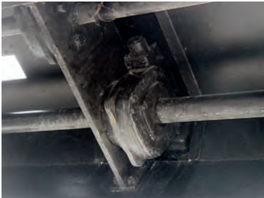
Figure 2.097: Centre mounted worm gearboxes turn two pinions each
