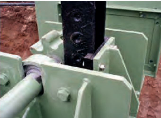
Figure 2.099: Secured connection thanks to a guide plate
