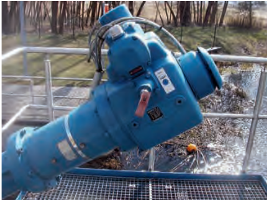
Figure 4.11: Absolute encoder on actuator of a lifting cylinder
