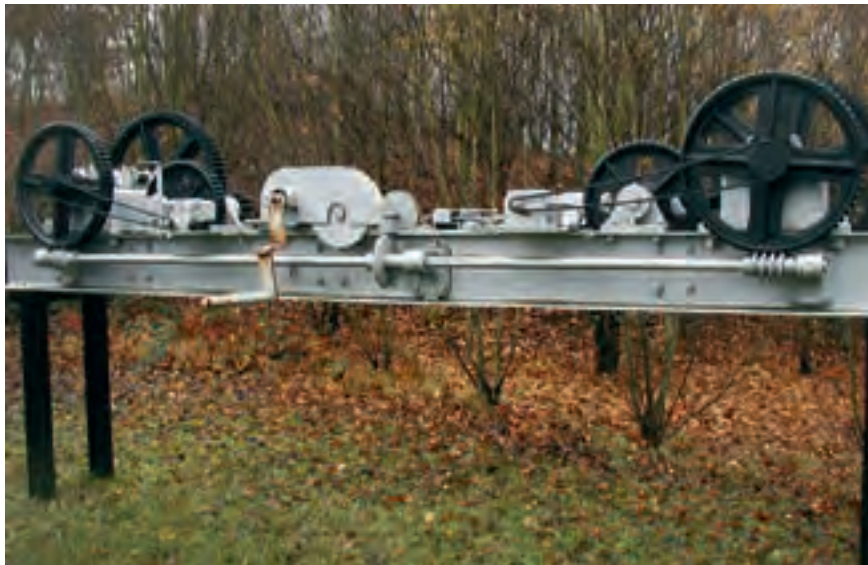
Figure 7.08: Manual drive for a double sluice gate with pinions and toothed racks
