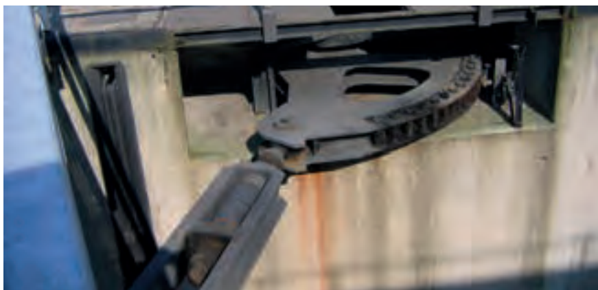
Figure 3.23: Slider crank gear with rounded lantern gear
