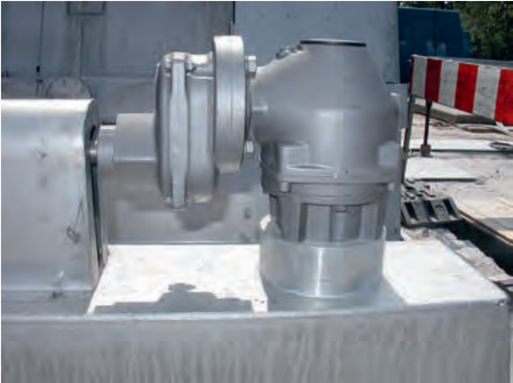
Figure 2.075: Reversing gearbox ahead of a bevel gearbox with spindle mount
