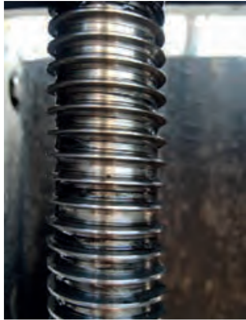
Figure 2.079: Strongly worn spindle within a narrow travel range
