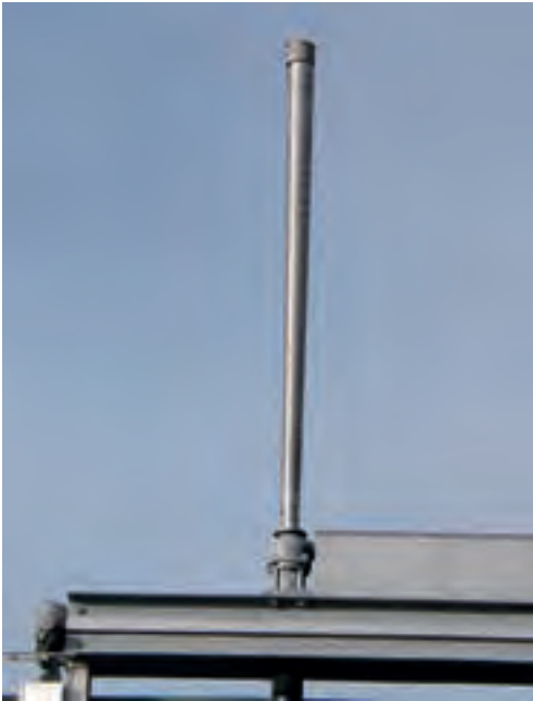
Figure 2.085: Risen spindle with extracted spiral protection and compressed bellows
