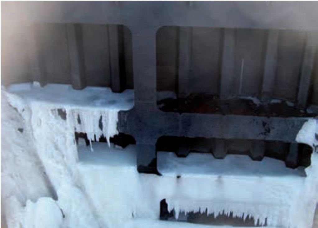
Figure 2.025: Applied ice load on cross bars
