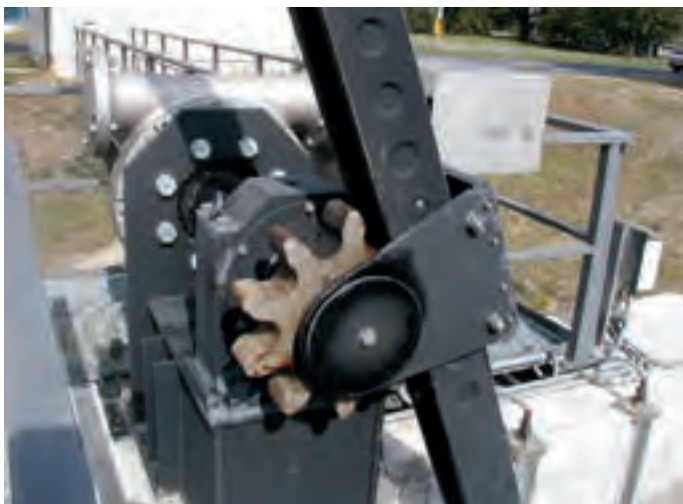
Figure 2.139: Pinion and lantern gear connected by buckle and buckle plate
