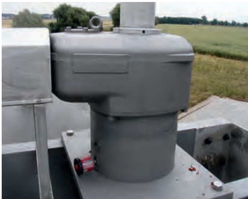
Figure 2.080: Bevel gearbox with A stem nut and lubricator
