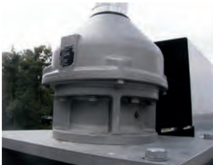
Figure 2.055: Bevel gearboxes with stem nut or spindle nut with lubrication point for bearings
