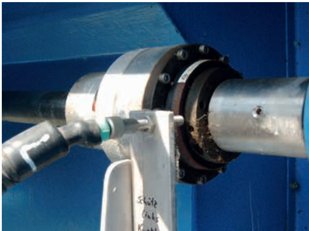
Figure 2.064: Slip clutch with proximity switches for electric tripping
