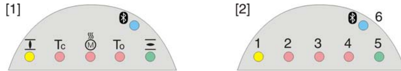
Figure 58: Arrangement and signification of indication lights
