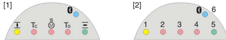
Figure 48: Arrangement and signification of indication lights
