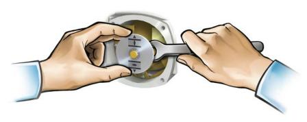
2. Refer to table and check if swing angle of the actuator corresponds to the setting of the reduction gearing (stages 1– 9).
