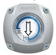
The self-adjusting mechanical position indicator shows the valve position by means of an arrow  $\Longrightarrow$ . When correctly set, the arrow points to symbol  $\blacksquare$  (OPEN) or  $\blacksquare$  (CLOSED) in the end positions.
