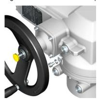
Figure 26: Earth connection for wall bracket
