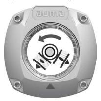
The mechanical position indicator shows the valve position via two indicator discs with symbols  $\blacksquare$  (OPEN) and  $\blacksquare$  (CLOSED). When correctly set, the symbols OPEN/CLOSED point to the indicator mark  $\blacktriangle$  at the cover in the end positions.
