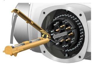
Pull fuse holder out of pin carrier, open fuse cover and replace old fuses by new ones.
