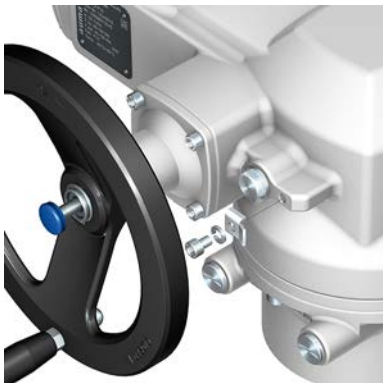
Figure 29: Earth connection for part-turn actuator
