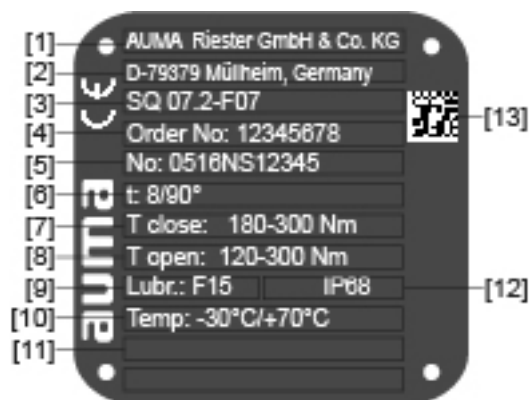
Figure 5: Actuator name plate (example)
