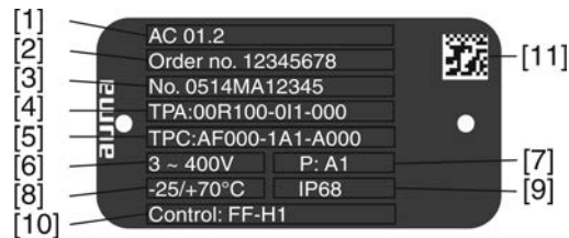
Figure 6: Name plate for actuator controls (example)
