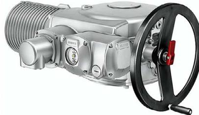
AUMA multi-turn actuators SA 25.1 – SA 48.1/SAR 25.1 – SAR 30.1 are driven by an electric motor and are capable of withstanding thrust in combination with output drive type A. For manual operation, a handwheel is provided. Switching off in end positions may be either by limit or torque seating. Actuator controls are required to operate or process the actuator signals.
