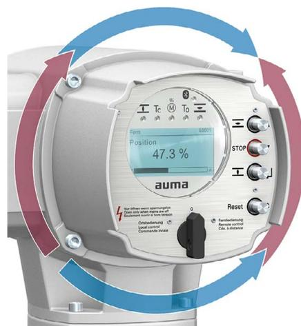
The mounting position of the local controls is implemented according to the order. If, after mounting the actuator to the valve or the gearbox on site, the local controls are in an unfavourable position, the mounting position can be changed at a later date. Four mounting positions shifted by respectively 90° are possible (by maximum 180° into one direction).
