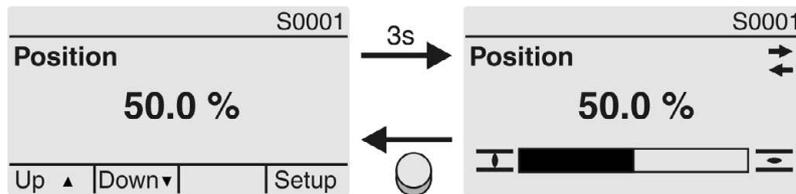
Reaching the preset end positions is additionally indicated via **⏏** (CLOSED) and **⏏** (OPEN) symbols.
