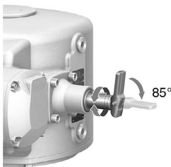
2. Push handwheel over the red change-over lever then onto the shaft.
