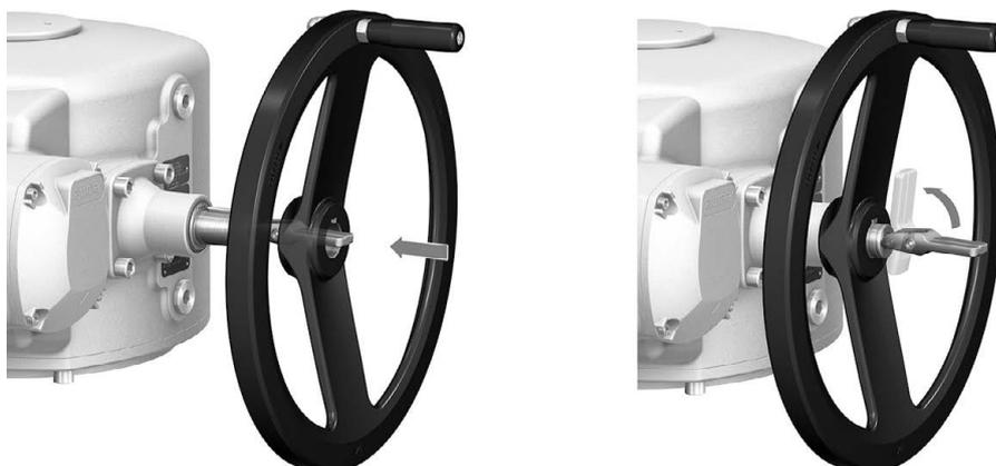
3. Release change-over lever (should snap back into initial position by spring action, if necessary, push it back manually).
