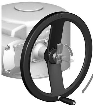
2. Release change-over lever (should snap back into initial position by spring action, if necessary, push it back manually).
